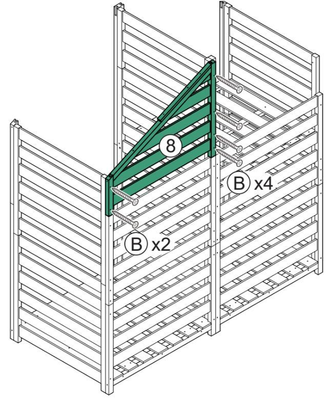
The diagram shows a wooden crate with a green diagonal slat (8) being inserted into the side panel. Six screws (B) are shown being driven into the slat from the right side to secure it to the frame.
