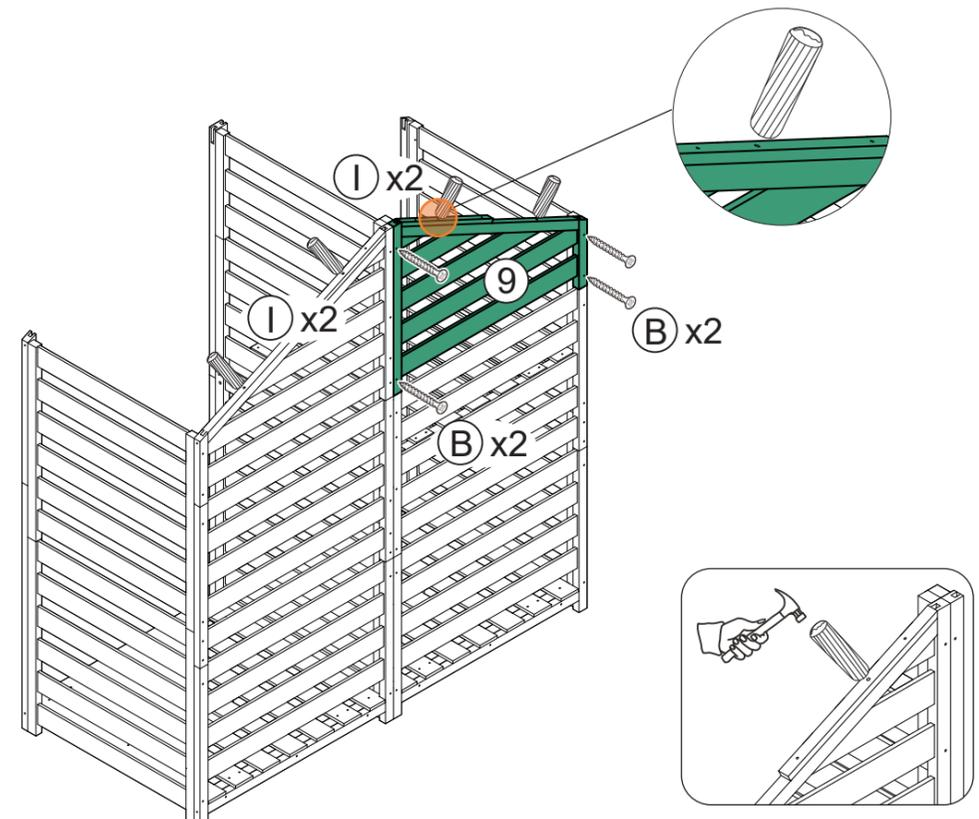
The diagram shows a wooden crate with a green diagonal slat (9) being inserted into the side panel. Four screws (B) and four nails (I) are shown being driven into the slat from the right side to secure it to the frame. A callout shows a nail being driven into the slat, and another callout shows a hand using a hammer to drive a nail into the slat.
