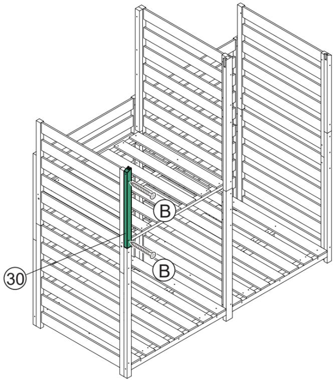
The diagram shows a wooden crate with a green vertical slat (30) being inserted into the side panel. Two screws (B) are shown being driven into the slat from the right side to secure it to the frame.
