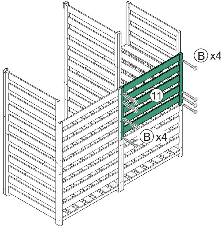
The diagram shows a wooden crate with a green horizontal slat (11) being inserted into the side panel. Four screws (B) are shown being driven into the slat from the right side to secure it to the frame.
