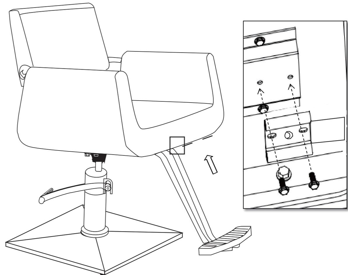
Please note that the foot rest and seat connection screws are pre- installed under the seat.
