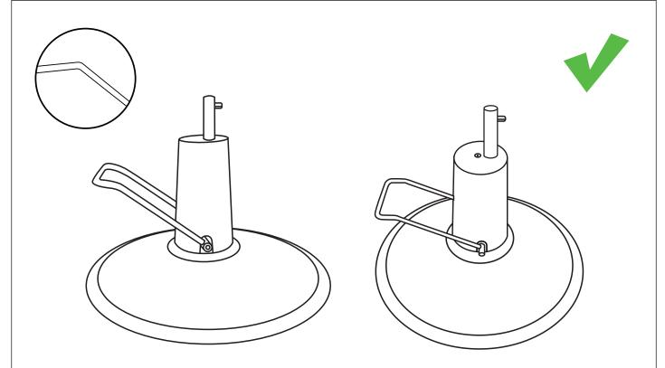
Please slip the foot lever through the pump rod. Please note that the curved part of the foot lever should be upward.
