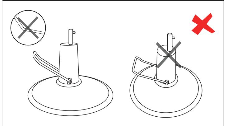
Please notice the direction of the foot lever and the insert direction when installing the foot lever.
