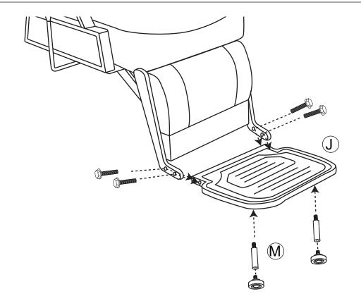
Please install the footrest and the legrest, and assemble the footnails under the footrest.
