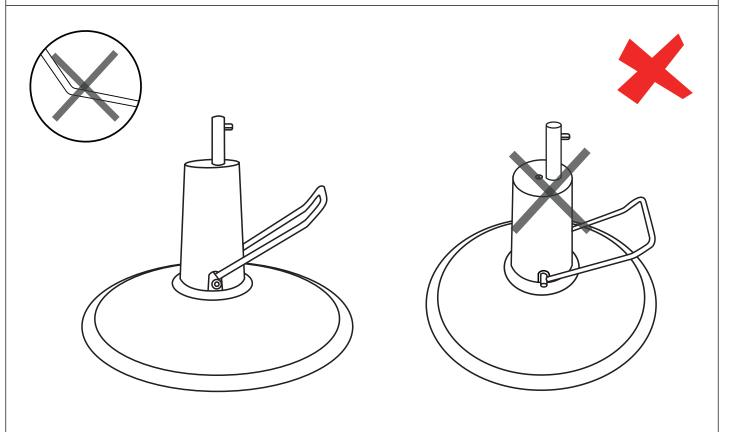
Please notice the direction of the foot lever and the insert direction when installing the foot lever.
