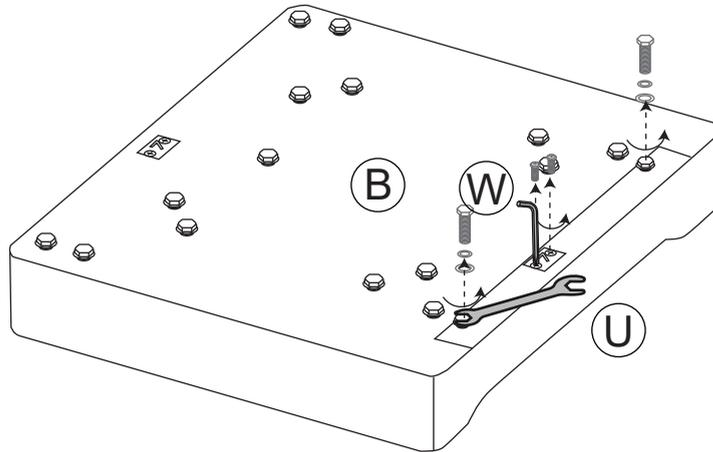
Place seat cushion (#B) flat on the ground, then use the open end wrench(#U) to unscrew the two hexagonal screws counterclockwise from the velcro. Remove the hex screws, flat washer, and spring washer.
