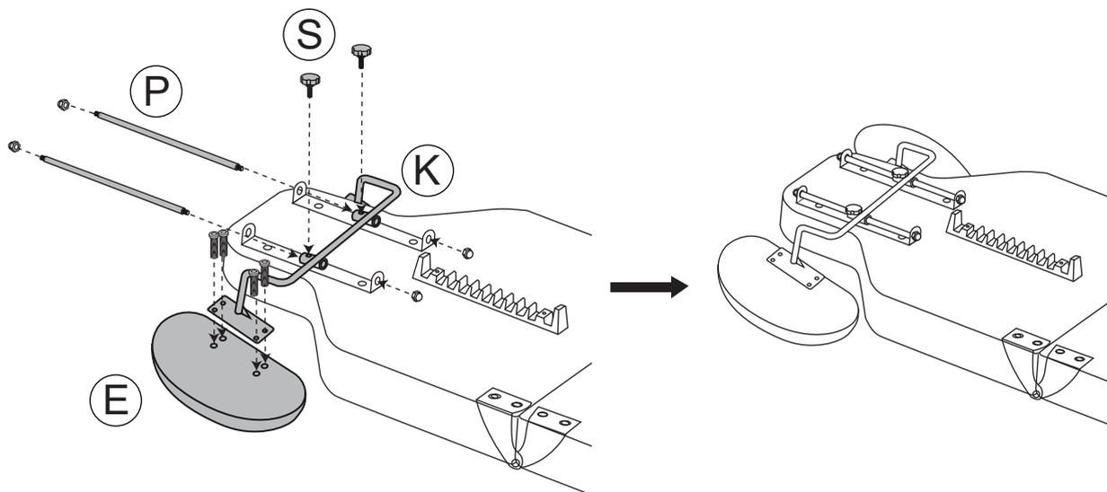
Unscrew the cover nuts on both ends of the sliding rod (#P), as shown in the figure below, and thread them through the fixing piece (#O) and the pillow holder (#K) in sequence. Use the cover nuts to tighten and fix them again, and install the knob (#S).
