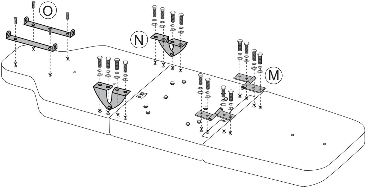
Unscrew the screws of the installation area for spare.
