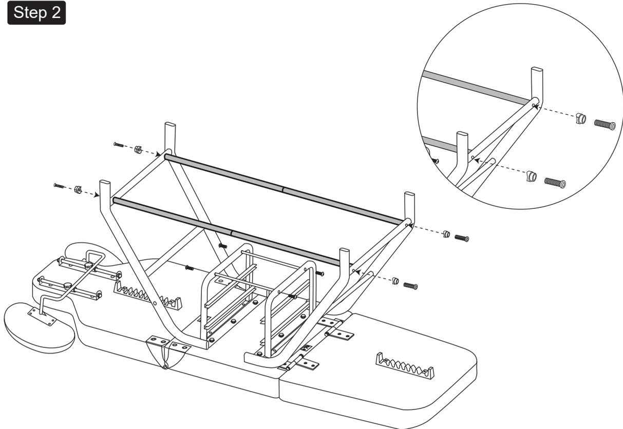
Align the two connected pipes with the installation holes at both ends of the bed frame, install the pipe sleeves, and tighten and fix them with screws, as shown in the diagram.
