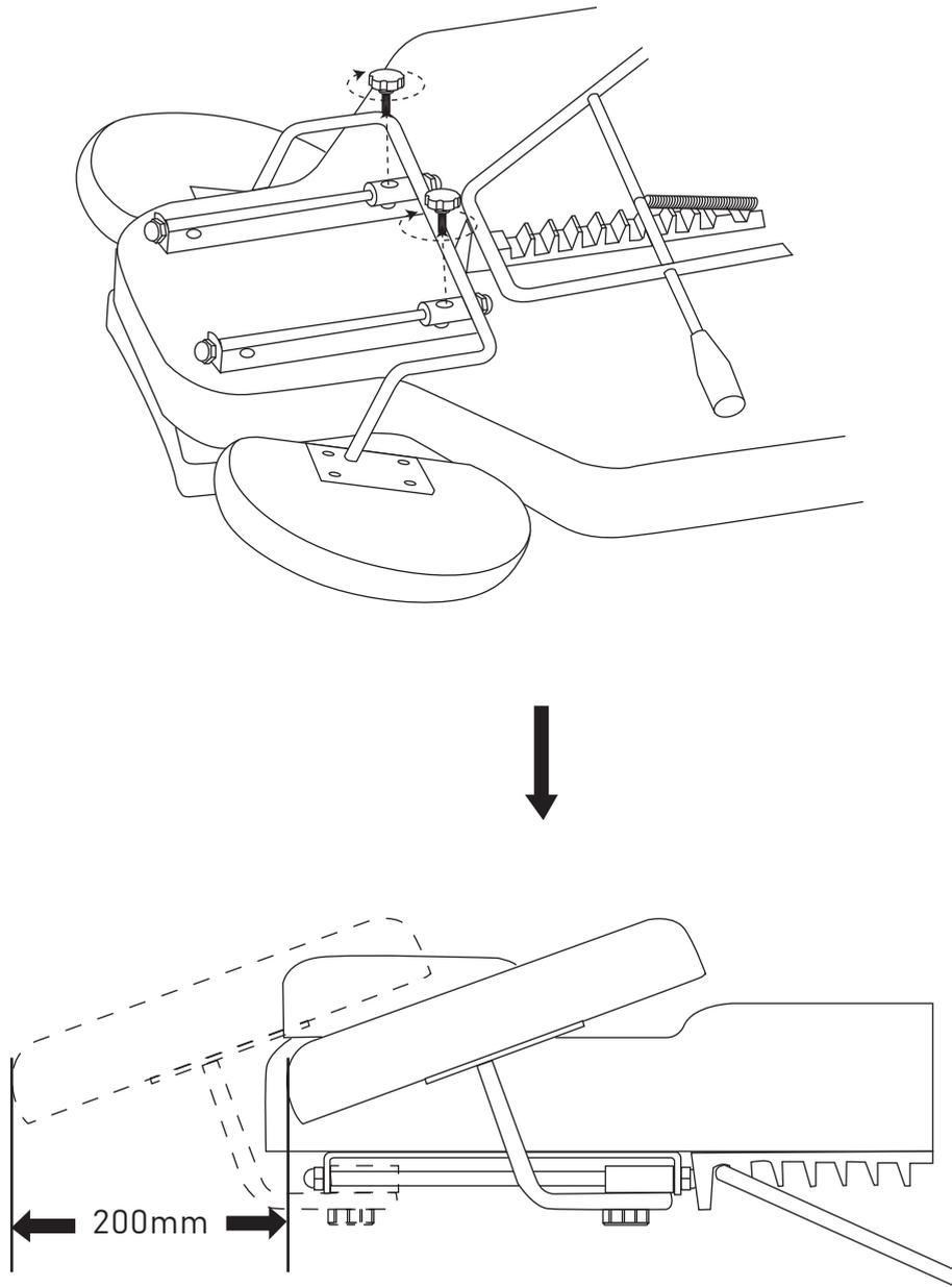
Release the knob to move the pillow, and tighten it clockwise to fix the position of the pillow, as shown in the diagram.
