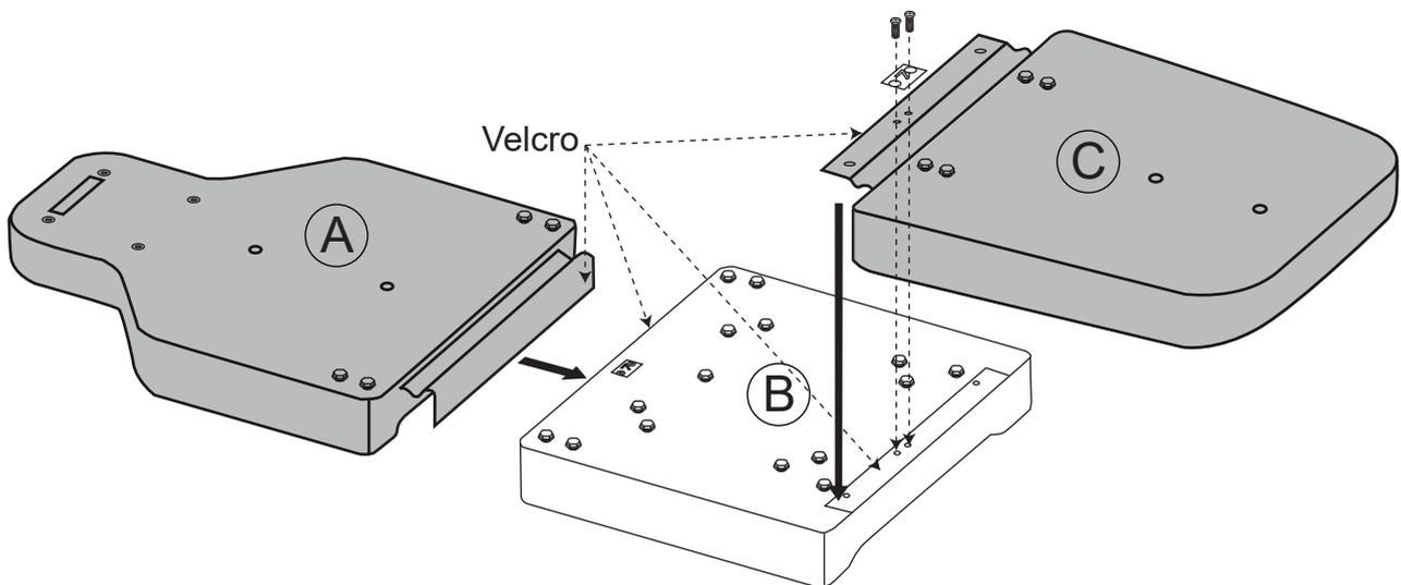
Arrange the backrest (#A), seat cushion (#B), and legrest (#C) as shown in the diagram, stick the velcro, and then tighten the spring hook with two cross screws.
