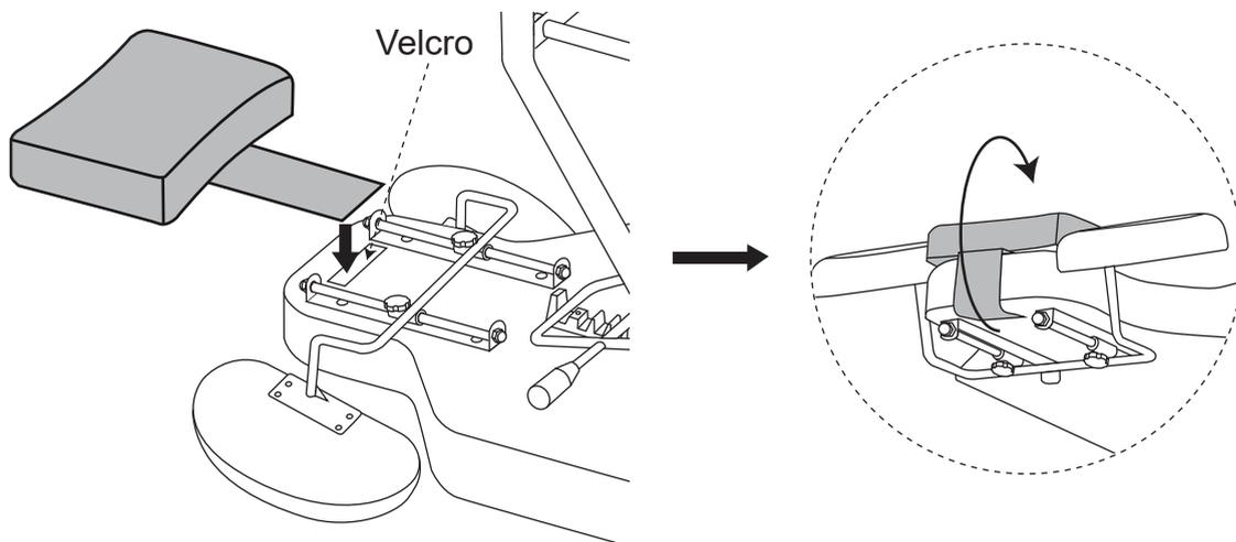
Glue the velcro on the headrest (#D) to the velcro on the back of the backrest (as shown in the picture), then flip the headrest over and place it on the backrest.
