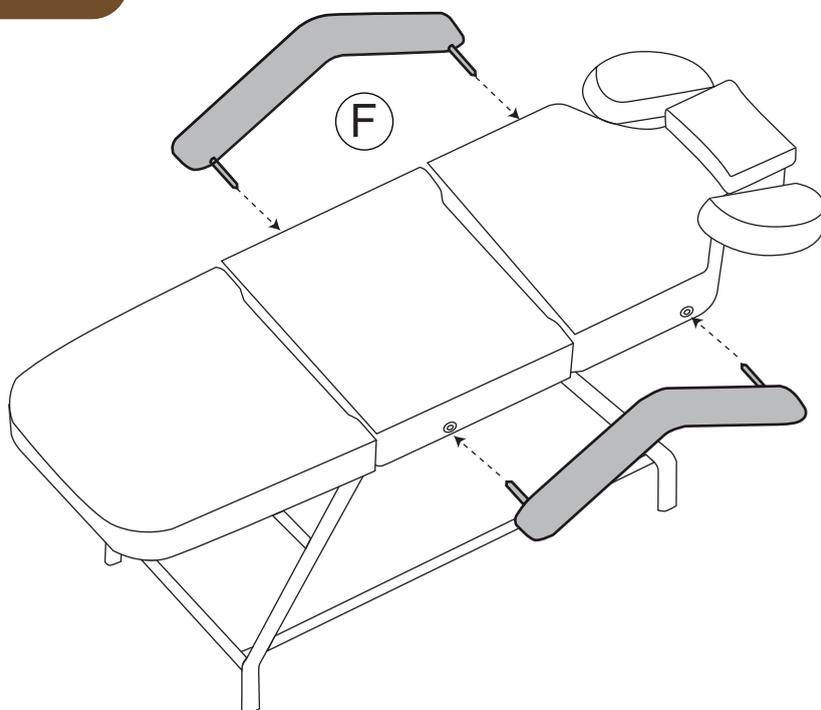
Align the connecting rod of the armrest (#F) with the installation hole on the left (right) side of the bed and insert it.
