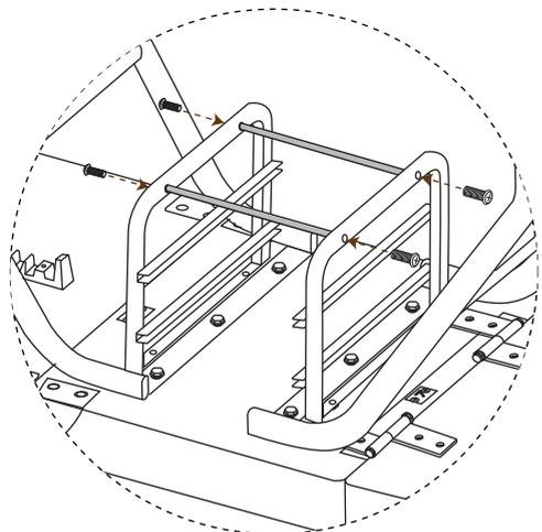
Unscrew the screws at both ends of the carriage connecting rod (#X), align them with the holes on both sides of the carriage frame (#J) as shown in the figure, and tighten the connection with the screws.
