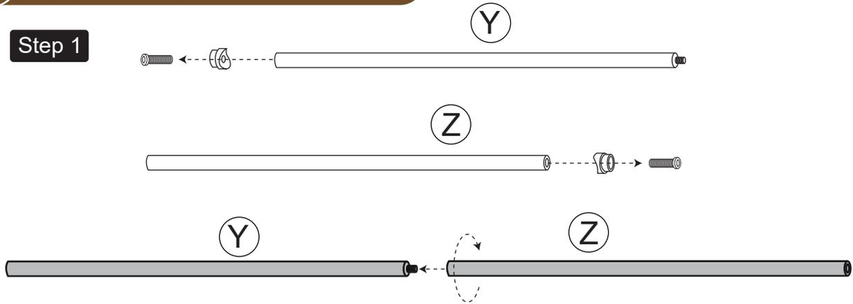
Unscrew the screws and pipe sleeves of the connecting pipe ① (#Y) and connecting pipe ② (#Z) for spare. Tighten connecting pipe ① (#Y) and connecting pipe ② (#Z) in a clockwise direction, as shown in the diagram.
