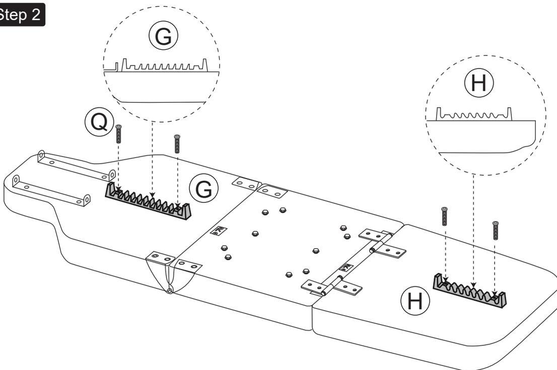
Use the M8x40 screws (#Q) from the tool kit to install the long ratchet bar (#G) and short ratchet bar (#H), paying attention to the installation direction, as shown in the diagram.
